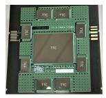
Recent testing by a large U.S.-based company has demonstrated the reliability of the TTV's from TEA, through 1000 cycles of -40C/150C thermal shock testing.
