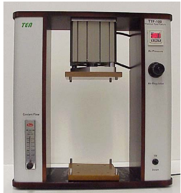
Standard air cylinder has 40mm diameter piston; optional 100mm diameter version is shown.
