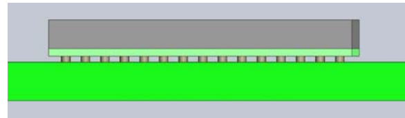
Figure 11b. Solder ball model representation
